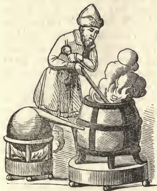
No. 185. Smelting ore with the blast of an Eolipile.
